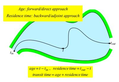
Nowadays marine models routinely produce large amounts of results. Making sense of all these real numbers is not a trivial task. This is why specific interpretation methods are needed. Estimating timescales is one of them. In this respect, a comprehensive theory (CART) is developed that allows for the estimation of timescales such as the age and the residence time from the solution of partial differential problems.
